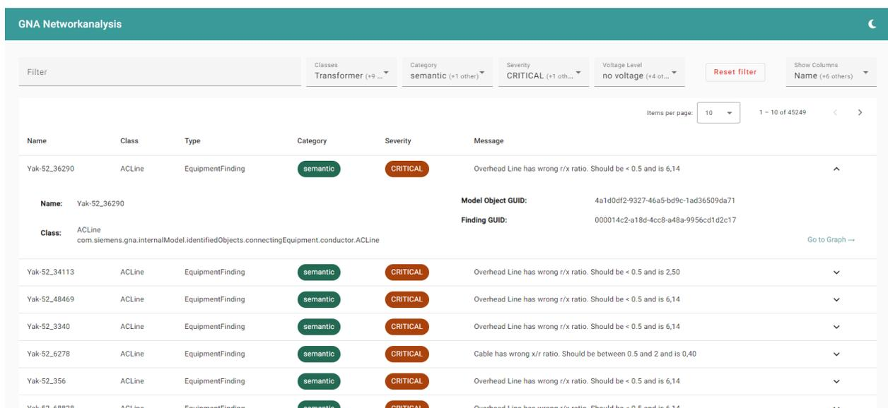
The screenshot shows the 'GNA Networkanalysis' interface. At the top, there are filter options for Classes (Transformer), Category (semantic), Severity (CRITICAL), and Voltage Level (no voltage). Below the filters is a table with columns: Name, Class, Type, Category, Severity, and Message. The first row is expanded to show details for 'Yak-52\_36290', including its Name, Class (ACLine), Model Object GUID, and Finding GUID.
