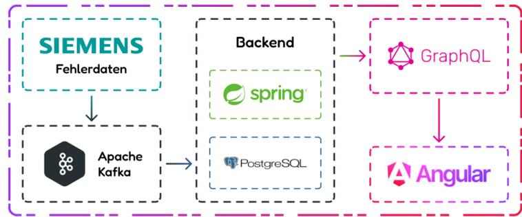
This graphic shows the architecture of our prototype. The data comes from the Siemens GNA and is stored in the PostgreSQL database through Kafka. From there, it can be retrieved by the frontend via a GraphQL API.
